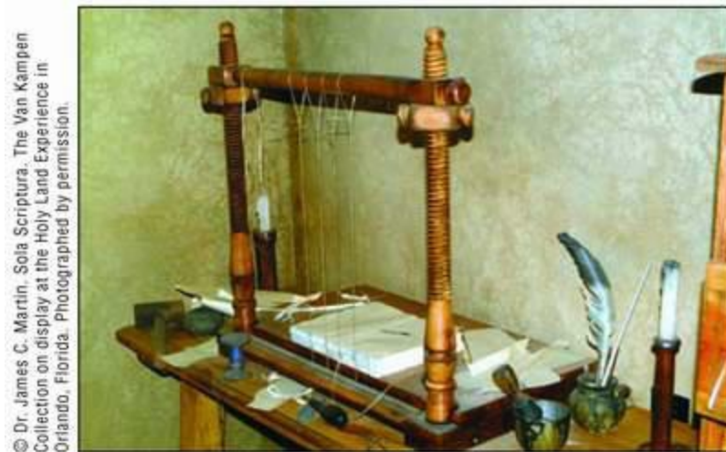
This tool is used to bind the pages of a book together when making a codex.
