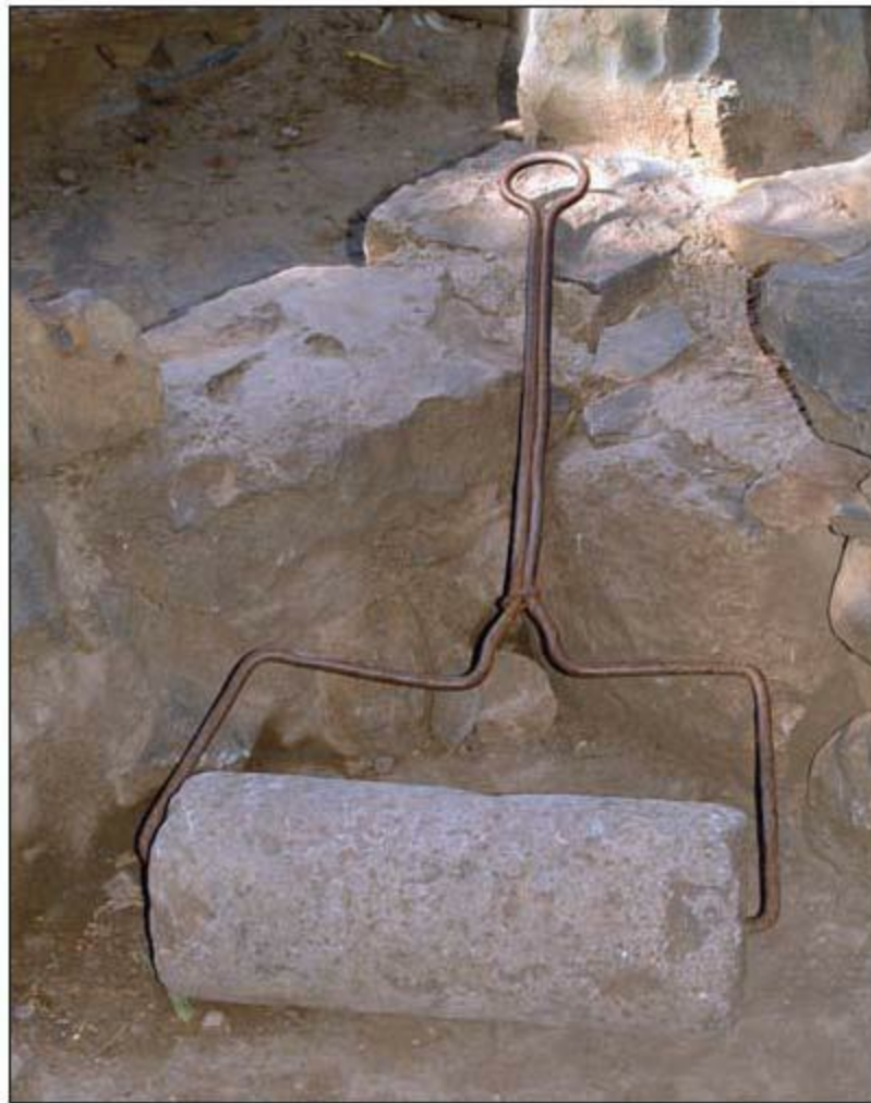
A basalt roof roller used to pack on mud thatched roofs of buildings.
