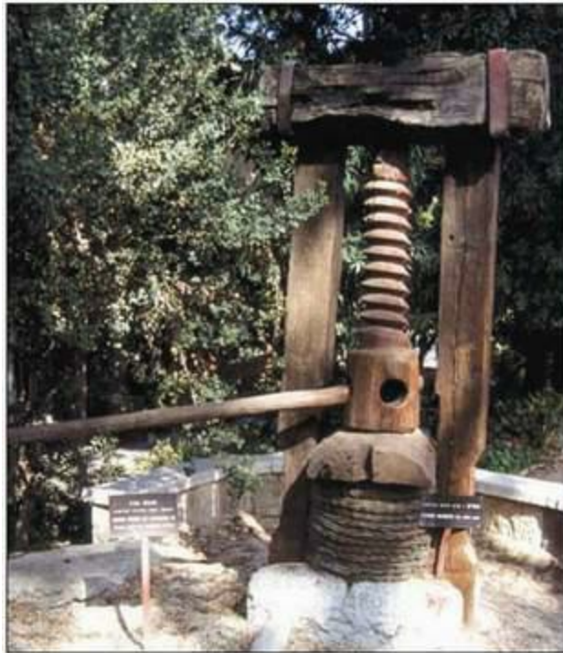
Wooden screw press used to extract oil from olives.
