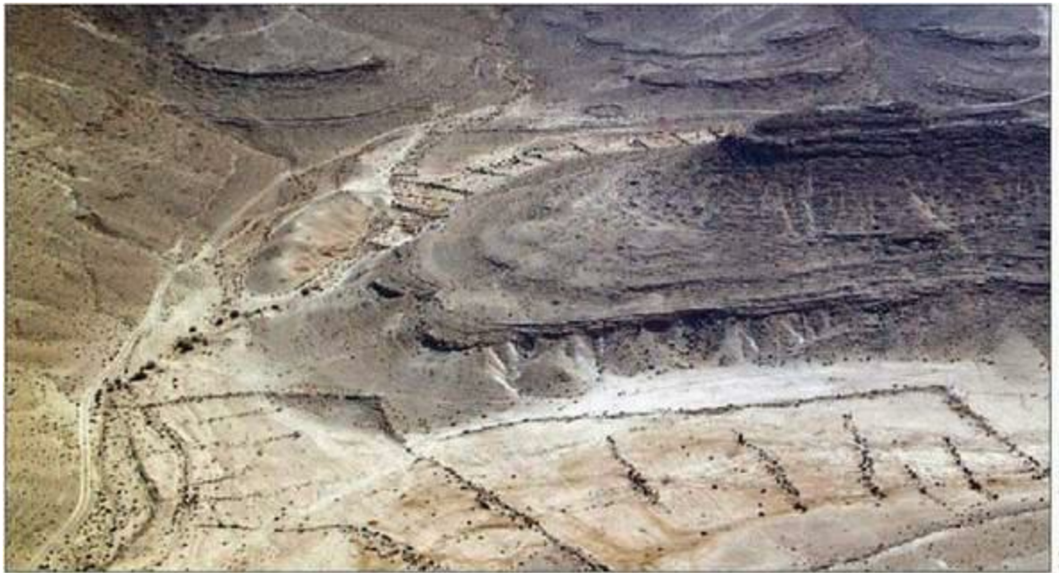
Aerial view near Ein Avdat along the Nabatean trade route from Petra to Gaza. In the foreground are stone walls located in the valley floor to slow the flow of water over the agricultural fields.
